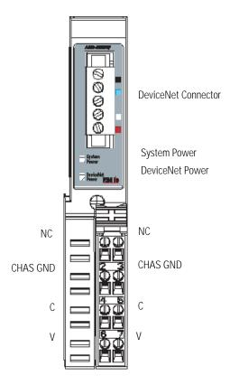
NC = No Connection CHAS GND = Chassis Ground C = Common V = Supply
