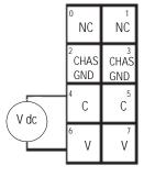
Connect this supply to the internal field-power bus.
