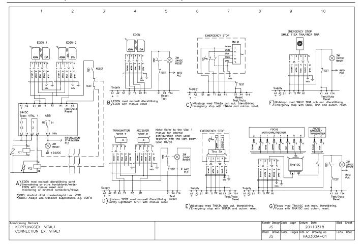
NB: If the safety light beam Spot 10/35 is connected to Vital 1, the information output switch must be in position 2. See section *Output connections* for further details.
