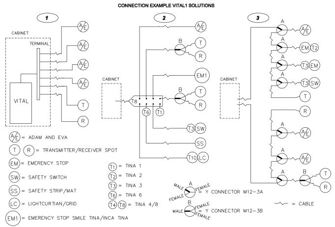
INFORMATION IS AVAILABLE VIA CABLE FROM EACH SENSOR IN EX.  $\overbrace{1}$  AND  $\overbrace{2}$
