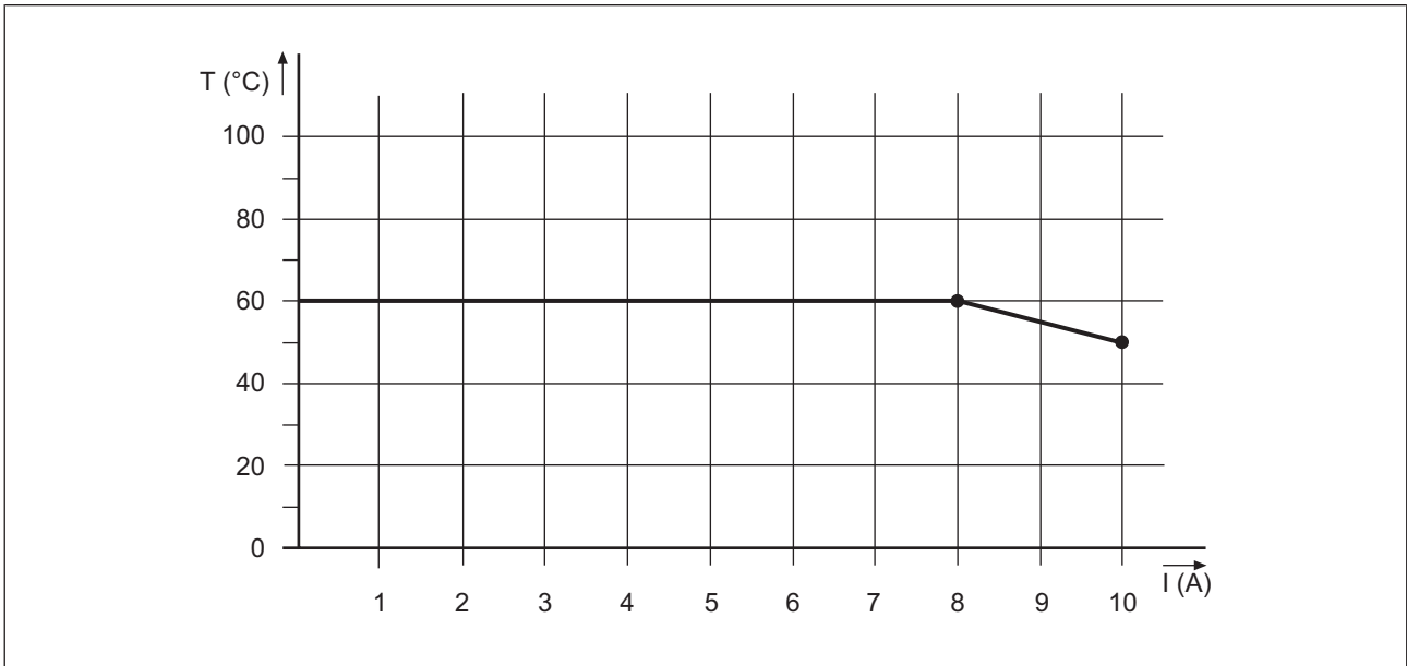
PSSu H FS SN SD(-T)(-R): Derating diagram for periphery supply: Permitted ambient temperature T dependent on load current I
