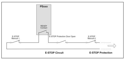
Figure 48: Power supply READY relay
