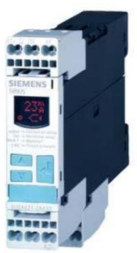
Digital monitoring relay Current monitoring, 22.5 mm from 0.05-10 A AC/DC 0vershoot and undershoot 24 to 240 V AC/DC 50 to 60 Hz DC and AC ON delay and noise pulses delay 0.1 to 20 s Hysteresis 0.01 to 5 A 1 change-over contact with or without fault buffer spring-type connection system
