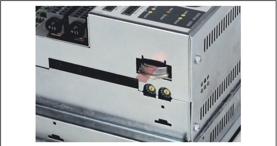
Figure 52: Power Panel 21 changing the battery
