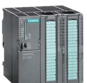
SIMATIC S7-300, CPU 314C-2 DP Compact CPU with MPI, 24 DI/16 DO, 4 AI, 2 AO, 1 Pt100, 4 high-speed counters (60 kHz), integrated DP interface, Integr. power supply 24 V DC, work memory 192 KB, Front connector (2x 40-pole) and Micro Memory Card required
