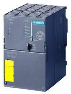
\*\*\*Spare part\*\*\* SIMATIC S7-300 CPU317F-2 PN/DP, Central processing unit with 1024 KB work memory, 1st interface MPI/DP 12 Mbit/s, 2nd interface Ethernet PROFINET, Micro Memory Card required Can be used with software package S7 Distributed Safety from V5.4
