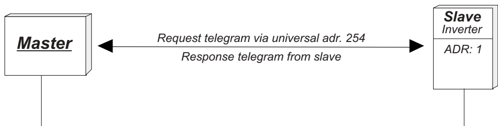
Fig. 16: Addressing in peer-to-peer connections with universal address 254
