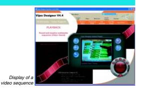
XBT GT terminals can be configured using the Vijeo Designer VJD ••D TGS V44M software, in a Windows environment. The evolutive ergonomics of the Vijeo Designer VJD ●●D TGS V44M software, designed around several parameterable windows, enables quick and simple development of a project. This version allows to manage the composite video signal from camera or camescope.
