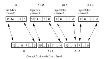
Analog output module, data type UINT16. mapping in the 3x/4x range
