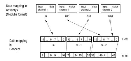
Analog input module, data type UINT16, mapping in the 3x range Addressing analog input modules for data type UINT16 is done using data mapping in the 3x/4x range according to the following illustration:
