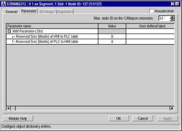
In the **Value** column, enter the word count that you would like to reserve in the Advantys STB Island for the communication of a Magelis terminal to the fieldbus master (HMI to PLC table) and for the communication from the fieldbus master to a Magelis terminal (PLC to HMI table). For the example, enter 9 words for each communication direction.
