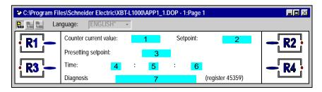
Field 1 Display counter current value from master (Concept register 401000)
