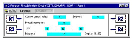
Field 1 Display counter current value from master (Concept register 401003)
