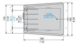
(1) 2 tapped entries for  $n^{\circ}$  16 (Pg 16) cable gland. For ISO M20, use adaptor DE9RA620.
